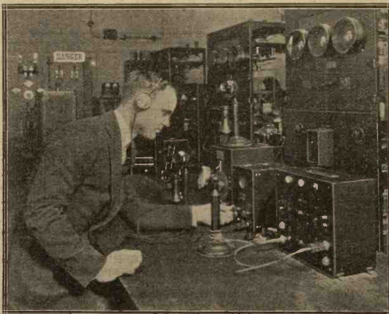
Listening for ship distress signals at Station WJZ. Every American broadcasting station must have a certified operator continuously on watch on 600 metres, (500 kc.), so that broadcasting can be stopped immediately an SOS call is heard.
